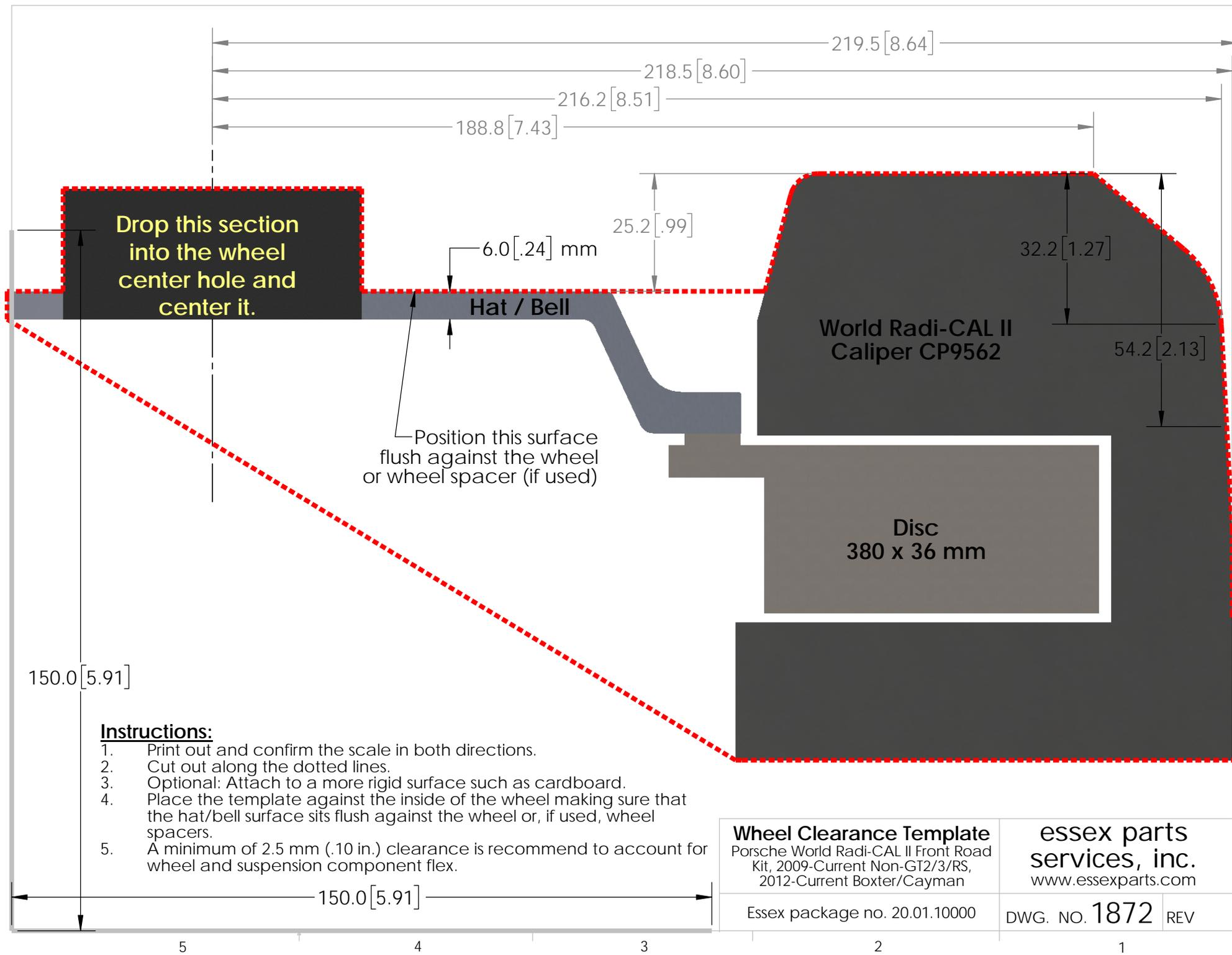
Drop this section into the wheel center hole and center it.
