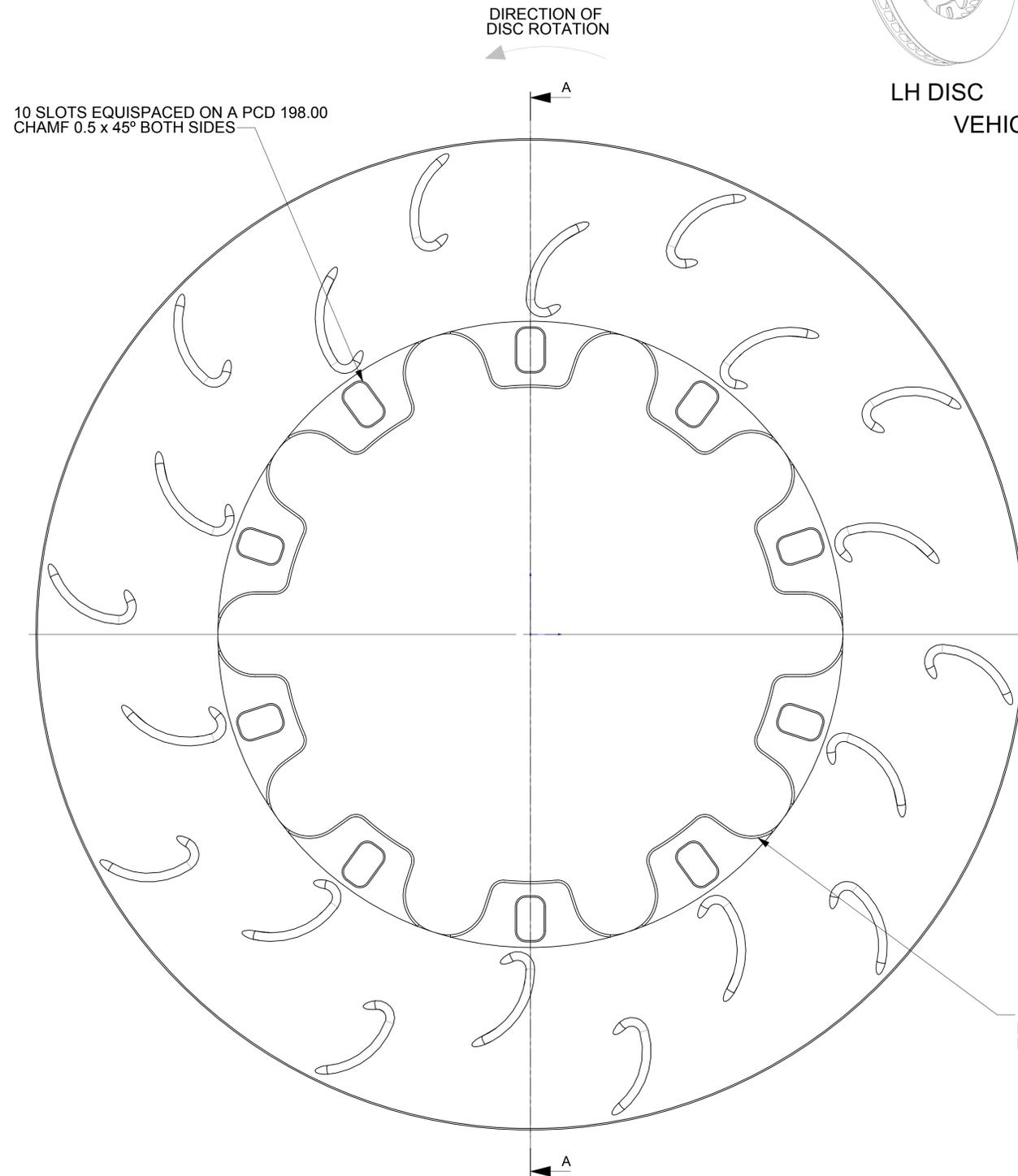
10 CUTOUTS EQUISPACED AND LOCATED CENTRALLY BETWEEN MOUNTING SLOTS AS SHOWN
