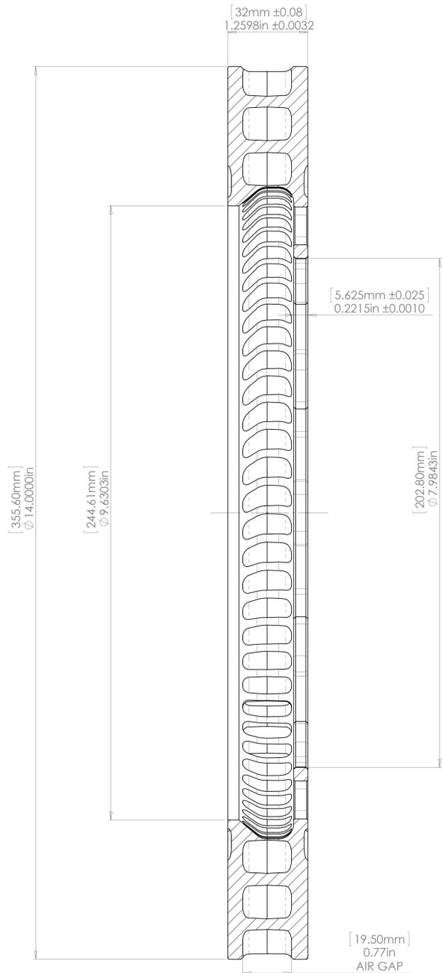
12 CUTOUTS EQUISPACED AND LOCATED CENTRALLY BETWEEN MOUNTING HOLES AS SHOWN.
