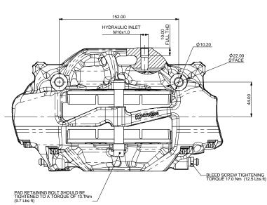
GENERAL DESCRIPTION THIS 4 PISTON DIFFERENTIAL BORE CALIPER TO SUIT UP TO Ø380 IRON DISC WITH A THICKNESS OF 28-32mm.
