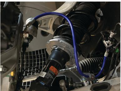
If line seems twisted, use the supplied plastic blocks and a pair of pliers to twist fitting so that the line is not overly twisted. See brake line packaging for instructions.
