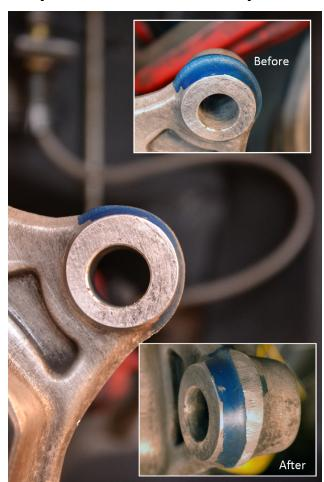
You can see in this picture (right) how the caliper bracket clears the spindle and sits flat against the machined surface.
