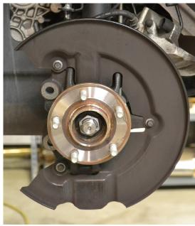
The Essex Competition brake system requires removal of the factory backing plate behind the OE disc in order to maximize wheel clearance. This plate significantly reduces the airflow into the disc center, so remving it will increase they system's performace. Using a 10mm wrench, remove the 3 bolts holding the plate onto the hub and discard.
