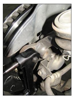
Using a 19mm socket/wrench and the supplied washers (#10.01.00100), attach the caliper bracket to upright in the orientation shown (Driver/Left side shown). The bracket has a small overhang on the caliper mounting surface that faces outboard. Be aware that the bracket is installed on the opposite face of the upright than the OE bracket. The left and right caliper brackets are identical for this application. Torque to 55 lb.-ft.
