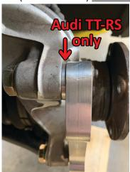
to upright (see picture on left). The left and right caliper brackets are identical for this application and include directions regarding their orientation in relation to the brake disc. Make sure that the bracket sits flat against the machined face of the spindle. **Torque to 105 lb.-ft** (142Nm).
