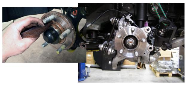
• The rear parking brake mechanism will be disabled with the Essex competition brake system.
