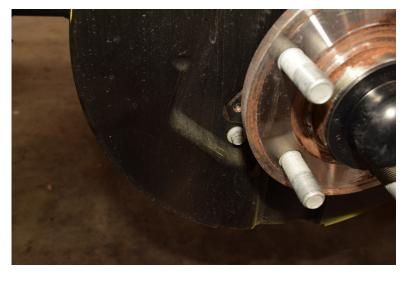
• Using a 10mm socket, remove the 3 bolts holding the backing plate to the spindle.
