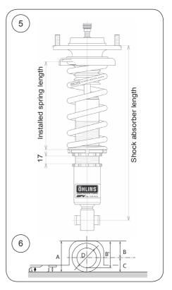
when compared to the original suspension. As the height adjuster is turned one rotation, the position moves 1.5 mm.
