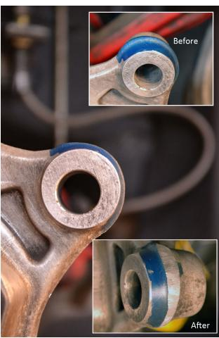
You can see in this picture how the caliper bracket clears the spindle and sits flat against the machined surface.
